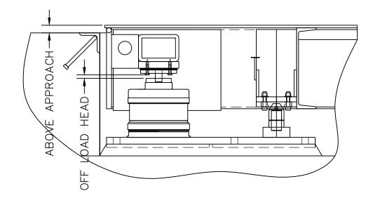
STEP 1: SLIDE THE REMOVABLE PINS DOWN OVER THE DOWEL PINS ON THE BASE PLATE. THE REMOVABLE PINS MUST SLIDE FREELY OVER THE DOWELS. SLOWLY AND CAREFULLY LOWER THE PLATFORM DOWN INTO THE PIT. KEEP THE PLATFORM LEVEL. THE REMOVABLE PINS MUST ALL PASS THROUGH THE CENTER HOLES IN THE CAPTURE BLOCKS.
