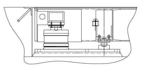
STEP 3: PULL THE REMOVABLE PIN UP THROUGH THE CAPTURE BLOCK AND STORE IT ON THE POST PROVIDED. THE SCALE IS READY FOR RECALIBRATION (AT THE DIGITAL INDICATOR).
