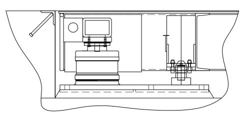
STEP 2: LOWER THE PLATFORM ALL THE WAY DOWN ONTO THE LOAD CELL. VISUALLY CONFIRM THAT THE LOAD CELL HEAD IS SEATED SQUARELY IN THE CENTERING RING.
