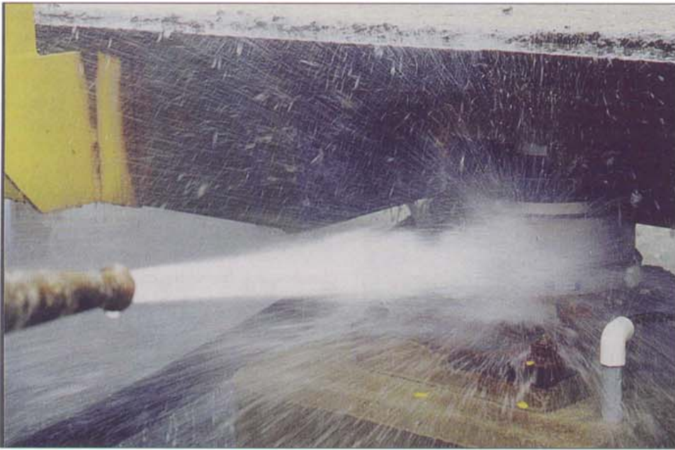
This load cell, under a hydrostatic truck scale, gets a direct blast from a high pressure hose.
