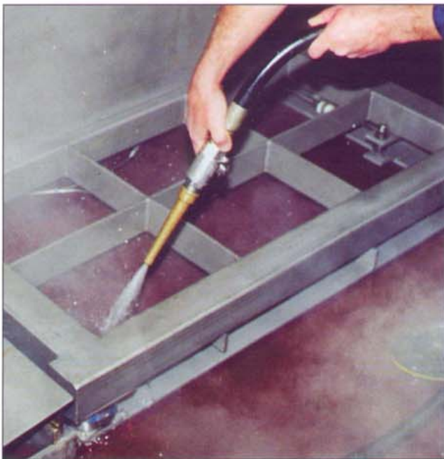
A hydrostatic load cell under a floor scale takes a direct blast from a high-pressure hose at a meat processing plant.
