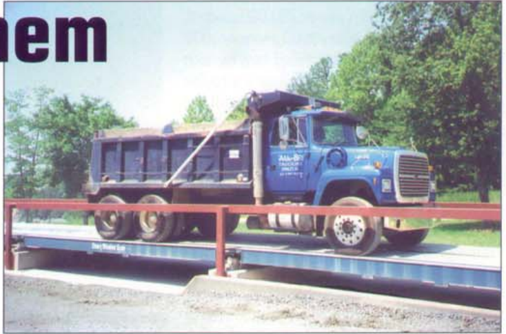
This above ground, steel deck Flat Top Truck Scale uses hydrostatic load cells. It is located at a quarry operation in North Carolina, and replaced a scale that was frequently damaged by lightning.
