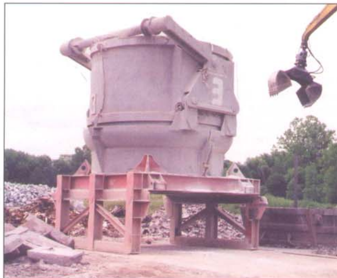
A scrap bucket at a steel mill is filled as it sets on a large 18- by 18-foot, 300,000-pound capacity pit scale.
