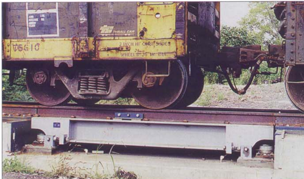
A pitless hydrostatic railroad track scale at a scrap company.
