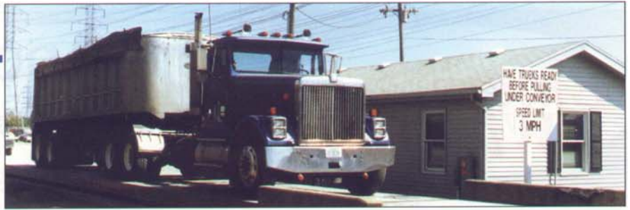
Seventy-foot hydrostatic truck scale serving wholesale fertilizer operations at The Andersons Inc.'s Delphi, IN. facility. Photo courtesy of The Andersons Inc.
