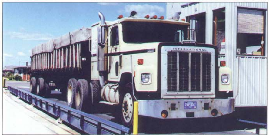
One of several hydrostatic trucks scales in service at The Andersons Inc.'s flagship elevator in Maumee, OH. This one is 93 feet long to handle full-size semis with pup trailers. Photo courtesy of Emery Winslow Scale Co.
