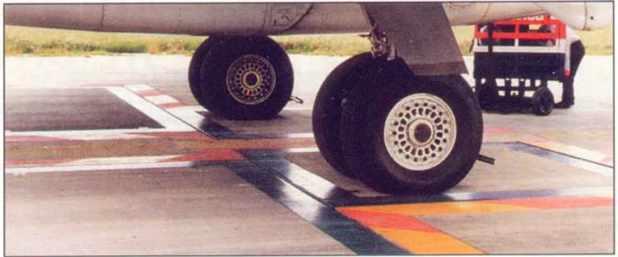
The AAWBVS installed at Bogota's airport consists of four main weighbridges with a reinforced concrete deck.
