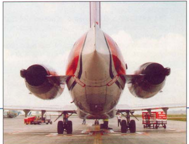
Aircraft positioned for weight and balance verification.
