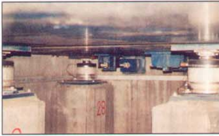
The AAWBVS installed at Bogota's airport consists of four main weighbridges with a reinforced concrete deck.
